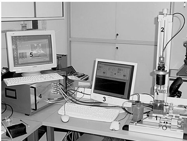
Fig. 1 Set up of the Hot Thermocouple Technique: 1 furnace chamber including heating units, 2 stand with camera and objective, 3 control PC, 4 control unit, and 5 PC for image recording
